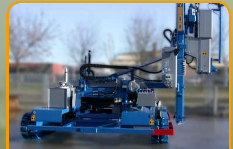
Hydraulically extendable crawler.
