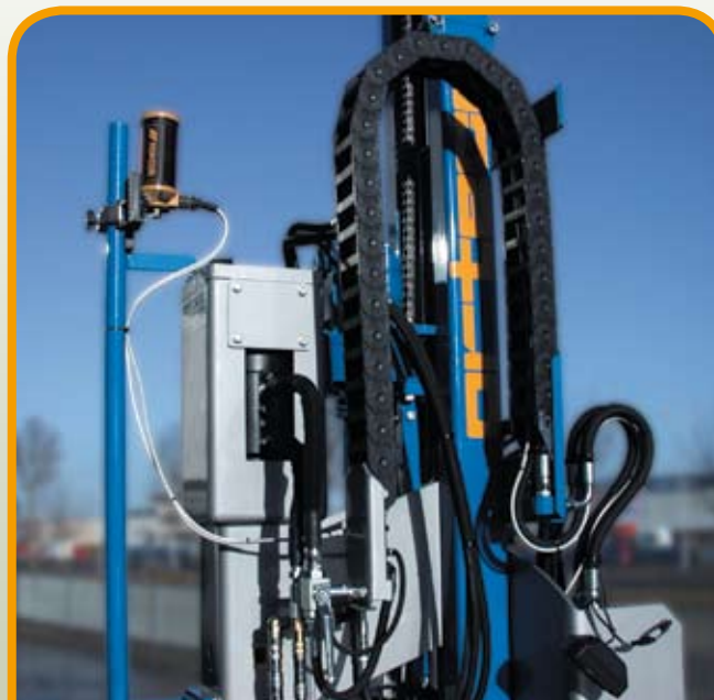
Active laser and auxiliary hydraulic circuit
