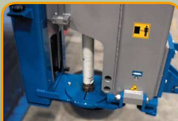
Down the hole hammer in stand-by position
